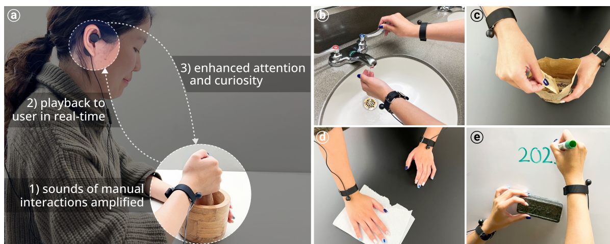
Fig. 1. (a) We propose a wearable device that amplifies sounds produced by ongoing hand interactions and plays them back to the user in real time, encouraging attention and curiosity toward the present-moment experience. The device supports mindfulness during everyday activities, such as (b) washing hands, (c) retrieving items from a paper bag, (d) cleaning a table, and (e) writing on a whiteboard. The figure is a posed demonstration of device use, with consent from the depicted individual.
